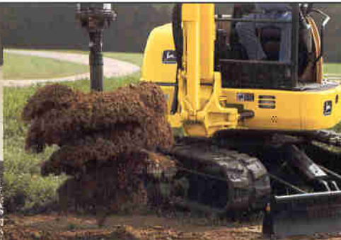
Hydraulic augers can be equipped with rock, heavy-duty, standard, and tree and shrub bits.
