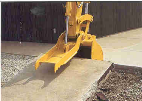
Add a hydraulic clamp and use it with the bucket for handling cumbersome objects.
