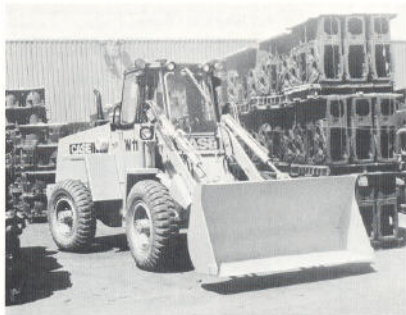
W11 equipped with .75 yd 3 (.57 m 3 ) bucket, cab, and 9.00 × 20 tires.
