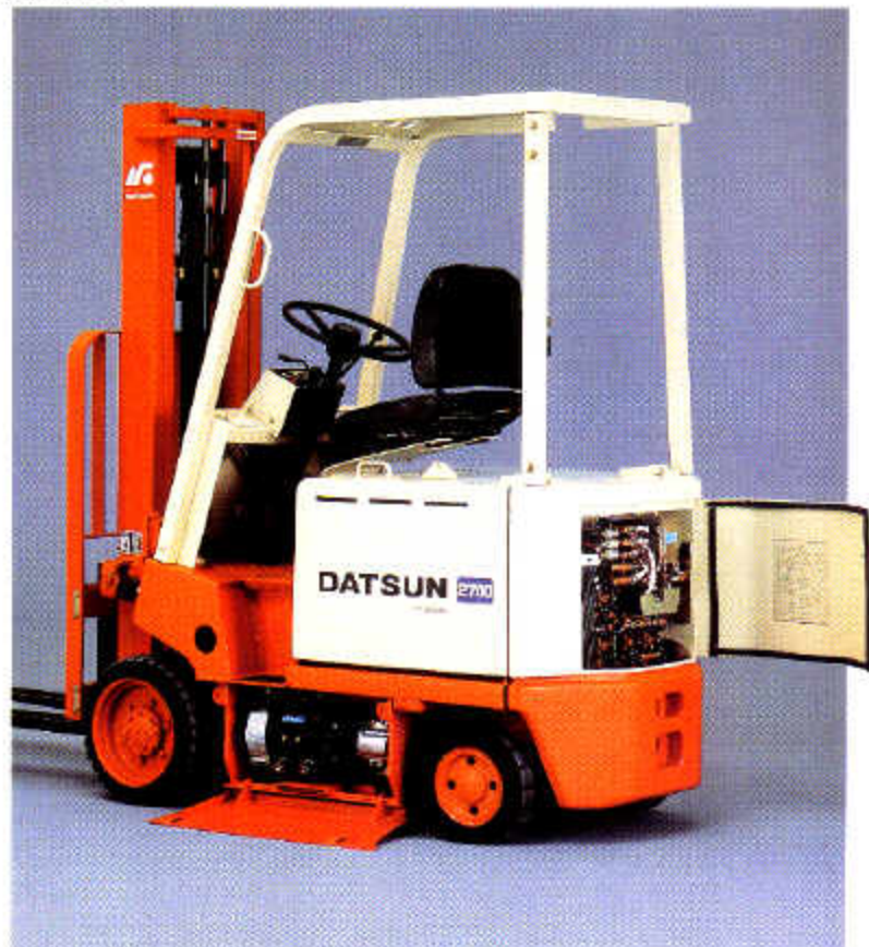
Easy-access controller and motors.
