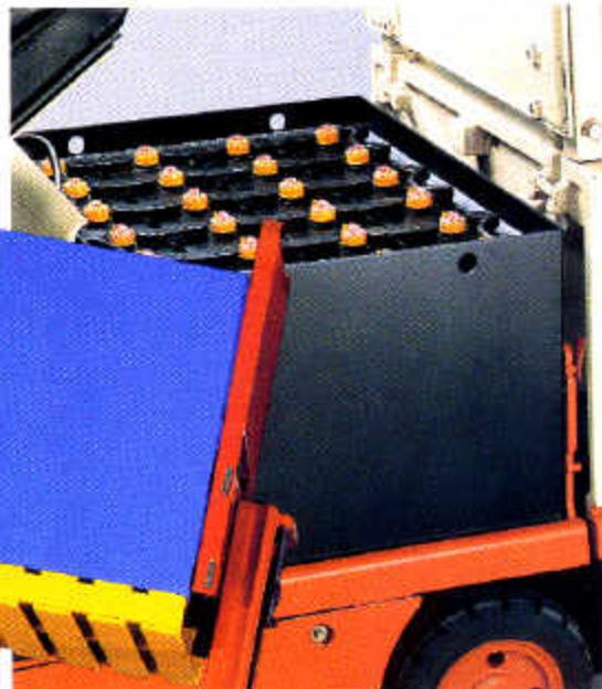
Large battery compartment.
