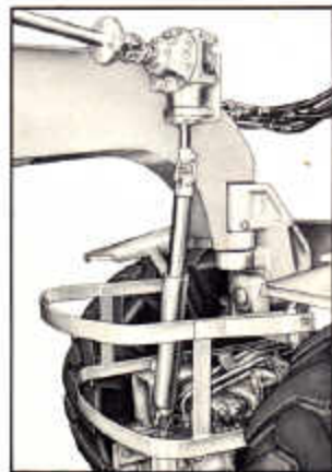
Detail of scraper-tractor mounting and 1000 rpm vertical PTO drive. No belts to wear out.
