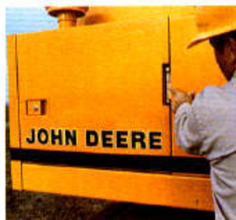
Sight gauge speeds hydraulic oil level check.
