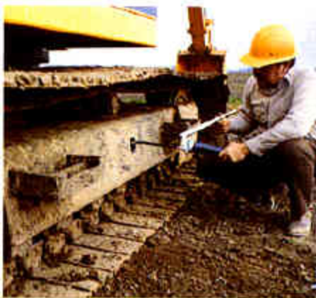
A grease gun is all it takes to maintain proper track tension, extending service life.
