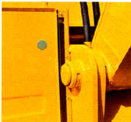
Fuel sight gauge near filler spout lets you check fuel level after locking cab at night.
