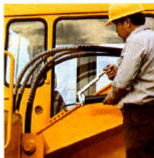
Central lube bank keeps you from climbing to grease elevated pin joints.
