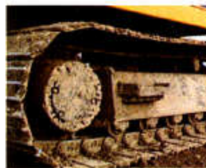
Permanently lubricated rollers, idlers, and large sprockets with floating seals extend durability, improve travel.
