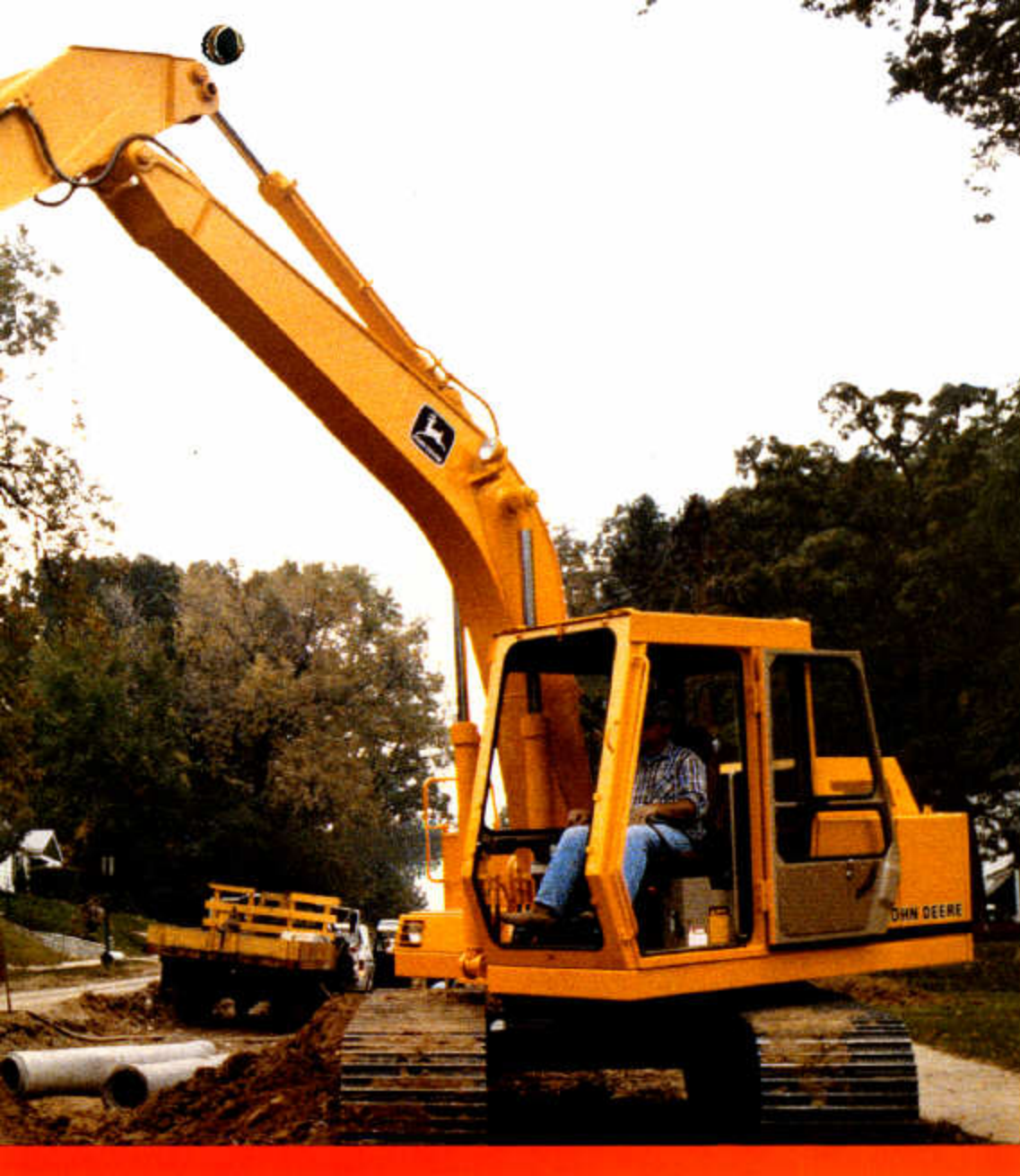
Permanently lubricated rollers, idlers, and large sprockets with floating seals extend durability, improve travel.
