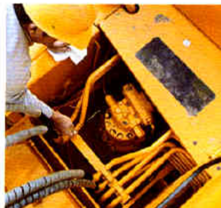
Swing gear oil level is easily checked from a non-skid platform.
