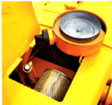
Air filter and engine oil may be inspected from one door on the hood.
