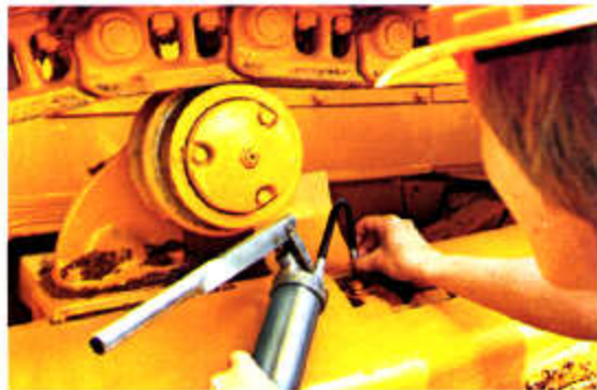
Make track adjustments with a simple grease gun.
