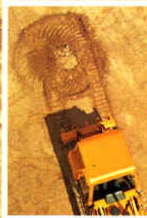
Independent counterrotating tracks increase maneuverability by allowing you to spot-turn the unit within its own length.
