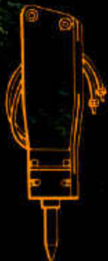
Hydraulic breaker busts rock, concrete, other hard materials. Useful where blasting is prohibited.
