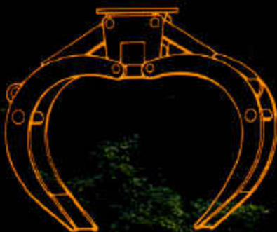
Grapples are available in different tine configurations for handling various materials.
